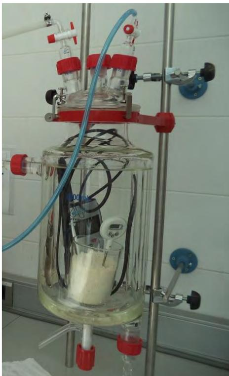
Figure 15. Reactor setup with the sensors inside.
