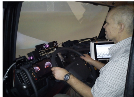
Figure 2: Positioning of iPad tablet and eye-tracking cameras in experimental set-up
