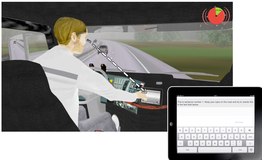
Figure 1: Positioning of the iPad tablet and eye-tracking cameras (capturing eye glance direction indicated by two yellow lines) in experimental set-up, driving scenario and drivers eye glance direction pointing off-road to the iPad tablet (white arrow)
