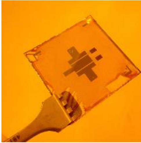
Figure 4-21: Picture of the four-cell module fabricated on a glass substrate.
