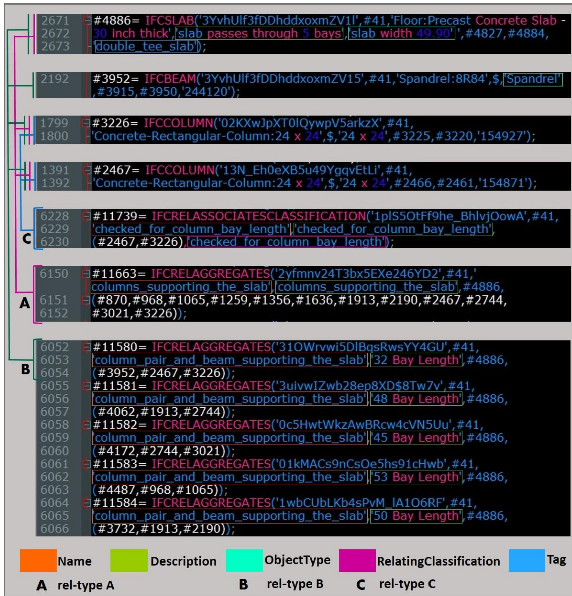
Figure 5.10: Collection of snapshots from an enriched IFC P21 file created by execution of the slab modularization rule set
