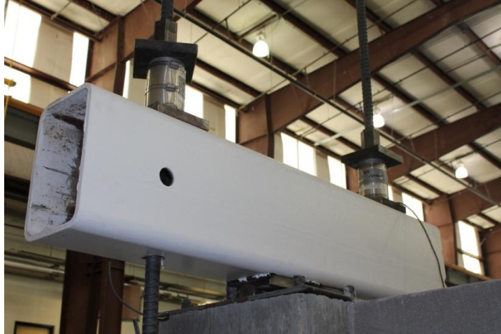
Figure 136: Load cells to measure column load throughout the test
