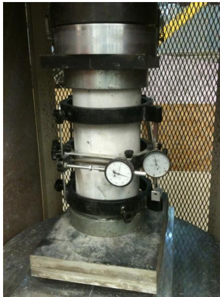
Figure 181: Test set up to determine the Elastic Modulus of concrete
