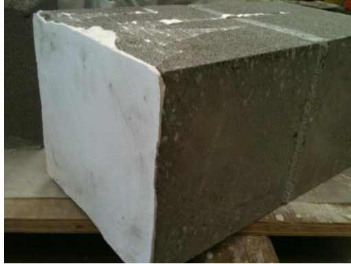
Figure 184: Gypsum plaster capping applied to all prisms
