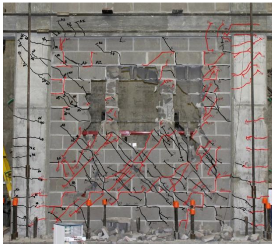
(a) Experimental Frame 1 (Full connection)
