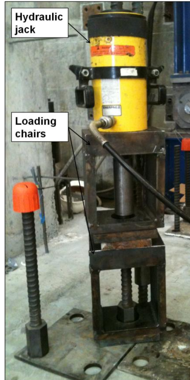
Figure 99: Post-tensioning slab to strong floor
