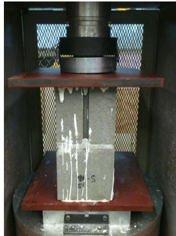
Figure 185: Test set up for compressive strength of masonry prisms
