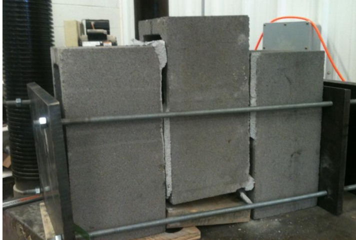
Figure 198: Failure of ungrouted triplet
