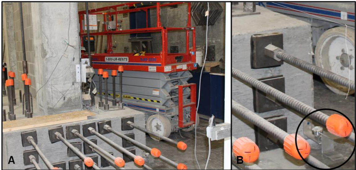
Figure 133: Lateral displacement of the columns measured by (a) string potentiometers accounting for (b) slip at the foundation
