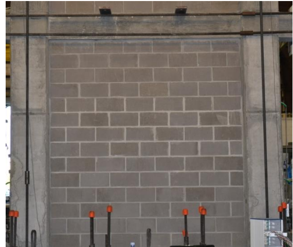
(b) Experimental Frame 2 (Connections only at the base)
