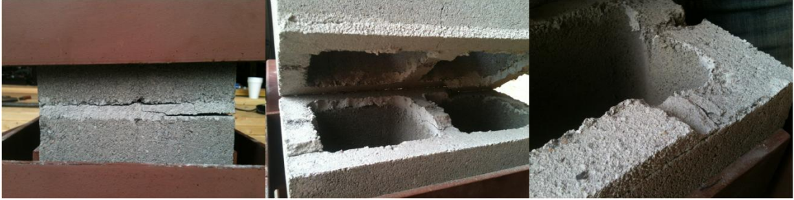
Figure 193: Failures of ungrouted bed joints
