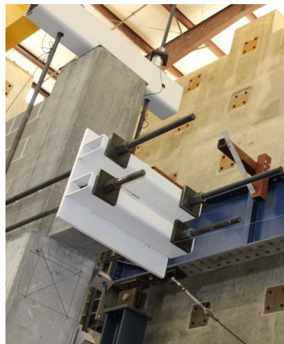
Figure 124: Stiffened plate on right side of loading cage
