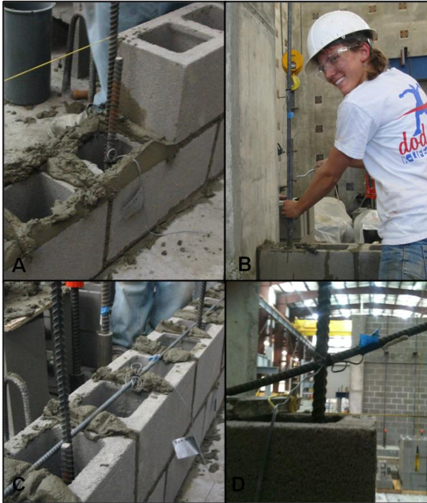
Figure 129: Strain gages in the masonry wall: (a) at base of vertical reinforcement, (b) at mid-height of vertical reinforcement, (c) at center of horizontal reinforcement, and (d) on dowel bars
