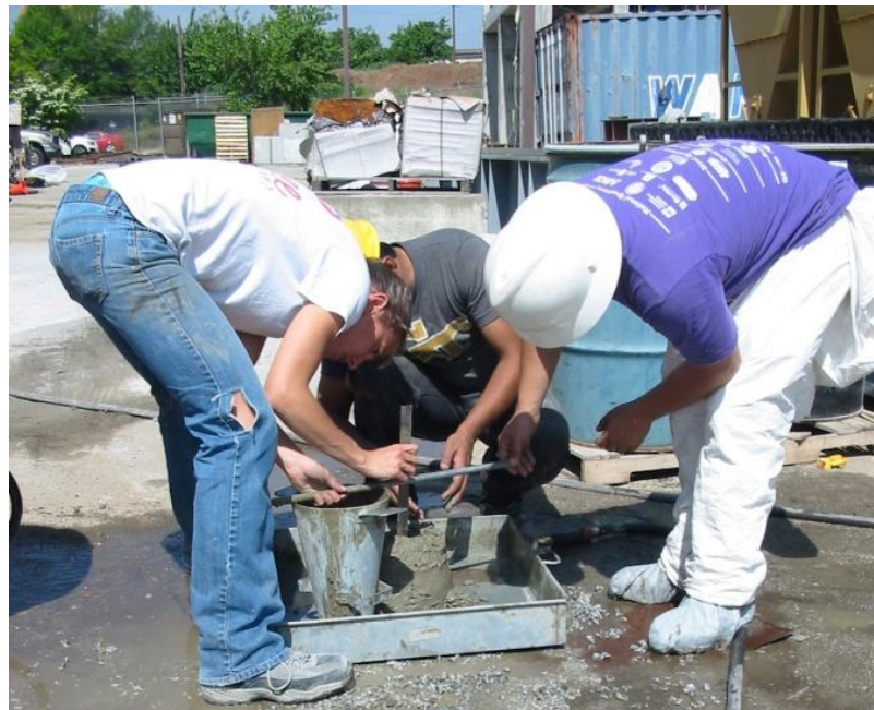
Figure 115: Measuring slump for weak concrete used to fill reinforced cells
