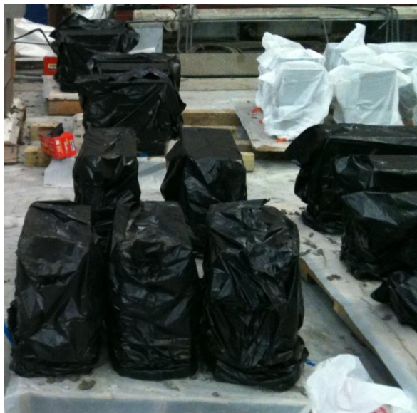
Figure 183: Prisms bagged for curing at ambient temperature
