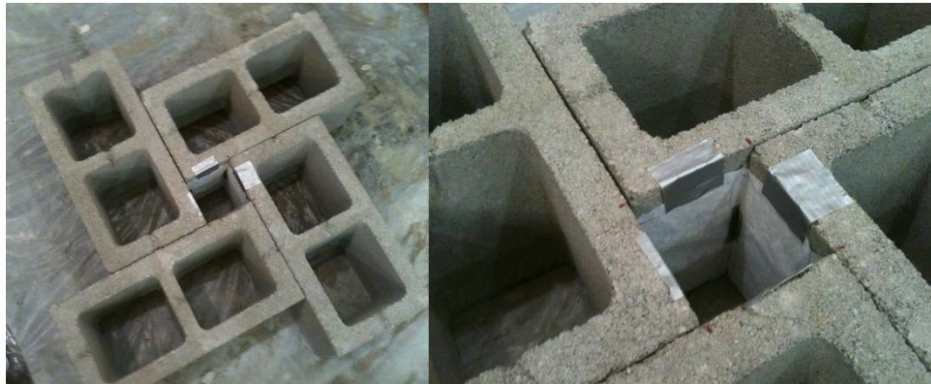
Figure 189: Grout cube mold as specified by ASTM 1019
