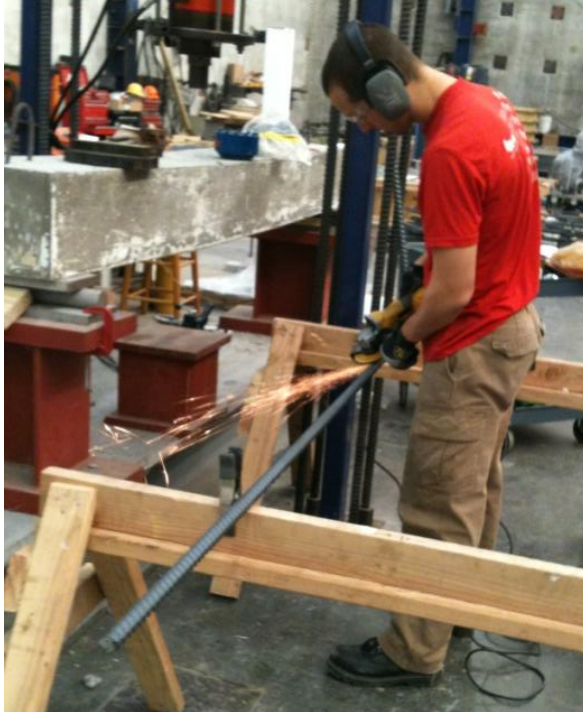
Figure 130: Grinding vertical column reinforcement to apply strain gages
