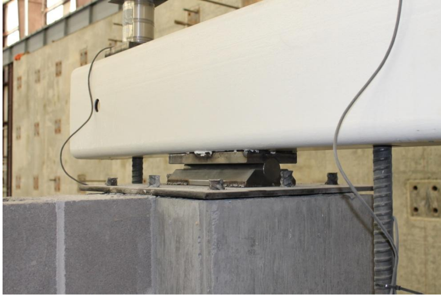
Figure 121: Column loads applied through transfer beam
