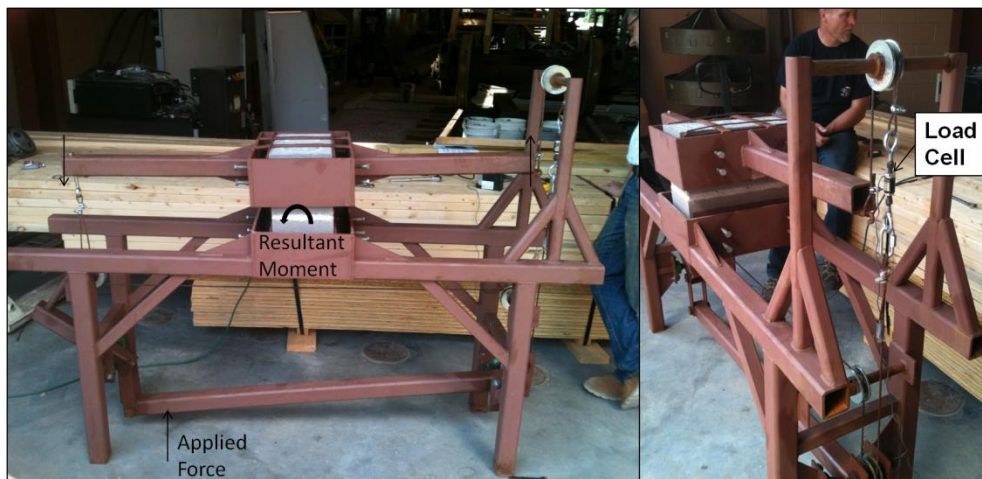
Figure 192: Bond wrench test set up
