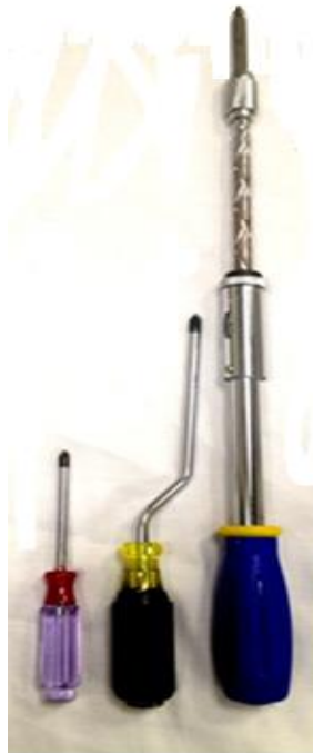
Figure 4.2: A familiar twist screwdriver, a rotational (plumber's) screwdriver, and a "Yankee" push screwdriver (from left to right).
