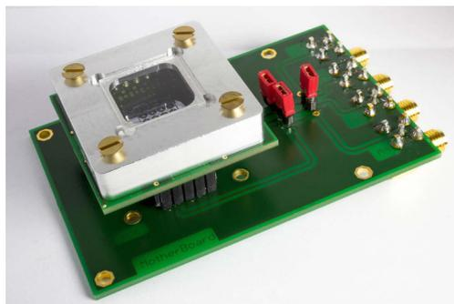
Figure 5.2: Protecting cap in aluminium with a transparent window on the top to allow optical characterisation.
