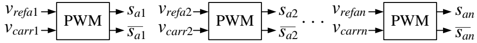
FIGURE 4.1: Phase a modulators having their own independent reference signal and their specific carrier.
