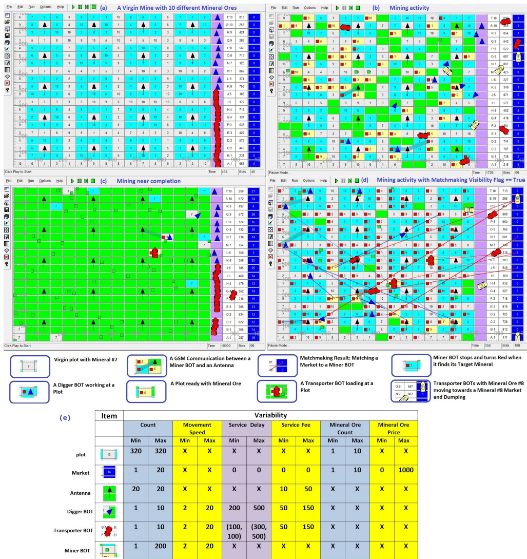
Figure 4.17: Above are a set of screen shots from the simulated experiments conducted on the "Mine Cloud" cloud robotic system. The Cloud in these experiments is simulated by the inter-agent message passing mechanism of the simulator. Part (a) above shows the virgin mine with 10 different kinds of mineral ores randomly embedded at 320 mine plots. The right-most column of the scene simulates the physical locations of the markets and corresponding columns in white displays their preferred mineral and the cost that they offer for that mineral at a given time. At the start of the simulation, all Digger and Transporter Robots are at their parking positions. Part (b) of the figure shows the mining action. Miner Robots search for their respective target mineral ores while Digger and Transporter Robots are hired by the Miner Robots at different stages of the mining process. The Transporter Robots loads the mineral ore from a mined plot and delivers the load to the market selected by the Miner Robot (Through the matchmaking mechanism). Part (c) shows a mine field near the end of the mining process. Most of the Miner , Digger and Transporter Robots are now free as very few mine plots remains to be mined. Part (d) shows the mining process with matchmaking associations made visible. At the peak of mining process, the number of matchmaking associations between agents could become very frequent. Part (e) is a table of various parameters that could be controlled for the simulated agent colony. It is necessary to have this variability in the simulation environment so that test cases with large variability could be formed.
