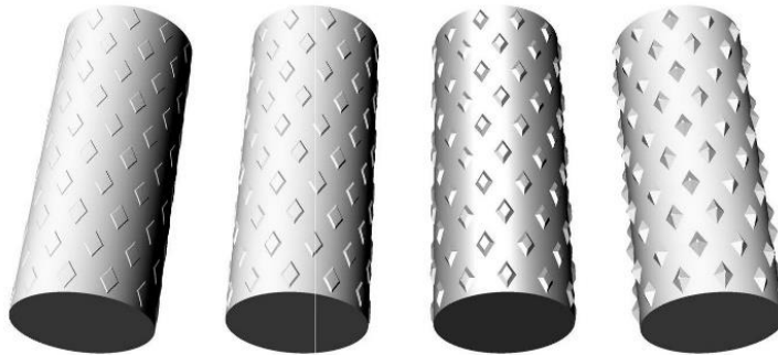
Figure 3.19: 3D rendering of friction sleeve of increasing surface roughness.
