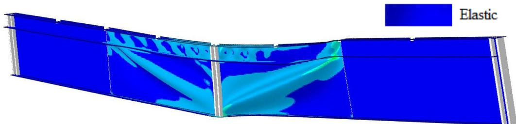
Figure 10-7: Typical failure mode for hybrid girder with high moment-high shear
