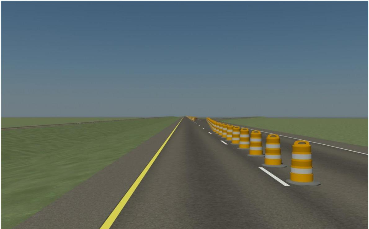
**Figure 3: Example Experiment 1 Rendering: Drums 10 ft. Apart, Ramp Open, Straight Freeway Alignment, 1 Second Travel Time to Diverge**
