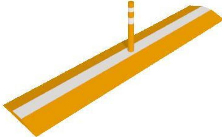
**Figure 6: Illustration of the Linear Channelizing Device used in Experiment 2. These segments would be placed end-on-end to create both closure and continuity.**
