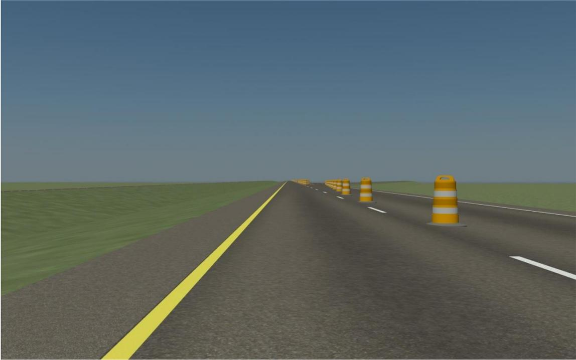
**Figure 61: Representative image of the D40A alternative. Image from Experiment 3, D40A alternative at 1 second distance in the straight geometry and the open condition with plain vegetation and no equipment.**
