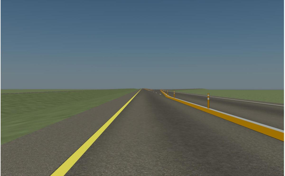
**Figure 4: Example Experiment 2 Rendering: LCD, Ramp Open, Straight Freeway Alignment, 1 Second Travel Time to Diverge**
