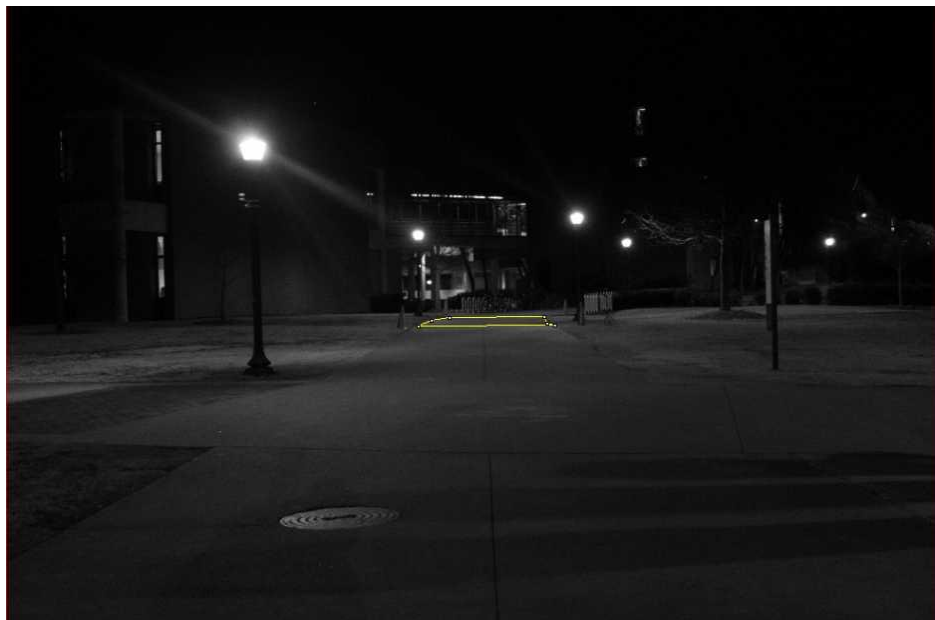
Figure 34 Concrete Walkway Test Site with the Luminance Measurement Area Highlighted in Yellow.
