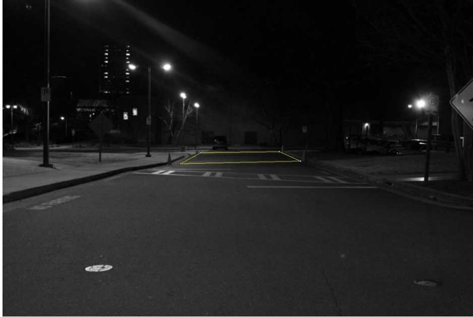
Figure 35 Asphalt Pavement Test Site with the Luminance Measurement Area Highlighted in Yellow.
