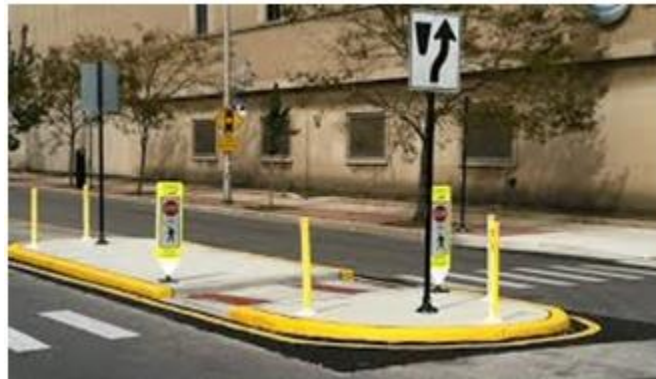
Figure D13 Example of a Refuge Island
