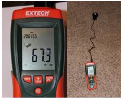
Figure C11 Picture of the EXTECH HD 450 ® Illuminance meter
