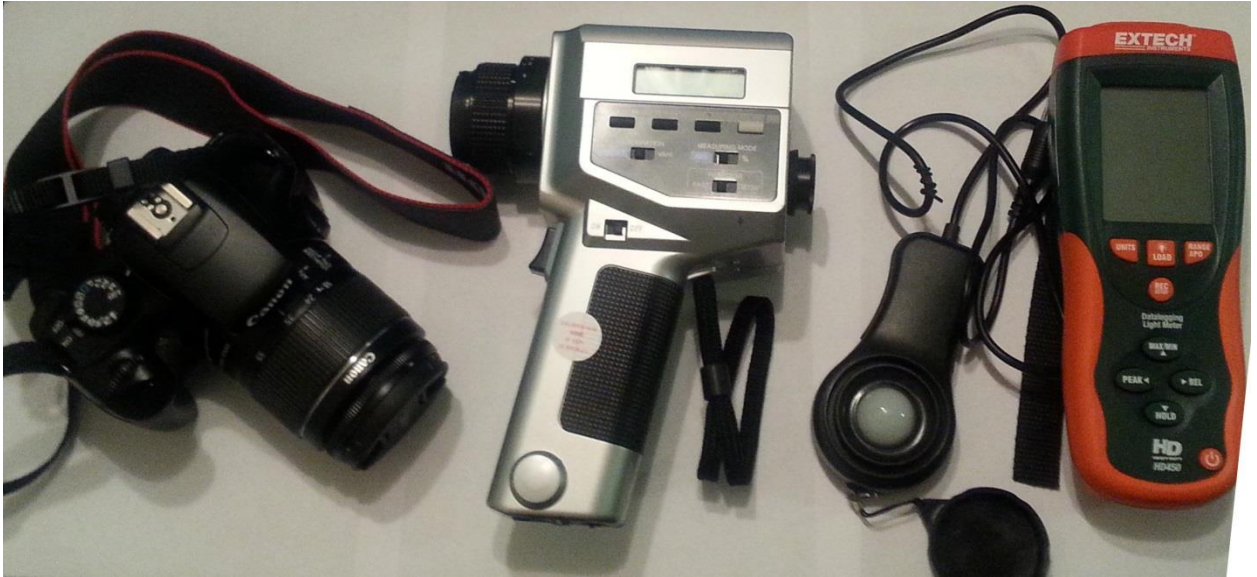
Figure 24 Digital Camera, Luminance Meter, and Illuminance Meter used for the Calibrating the Camera.
