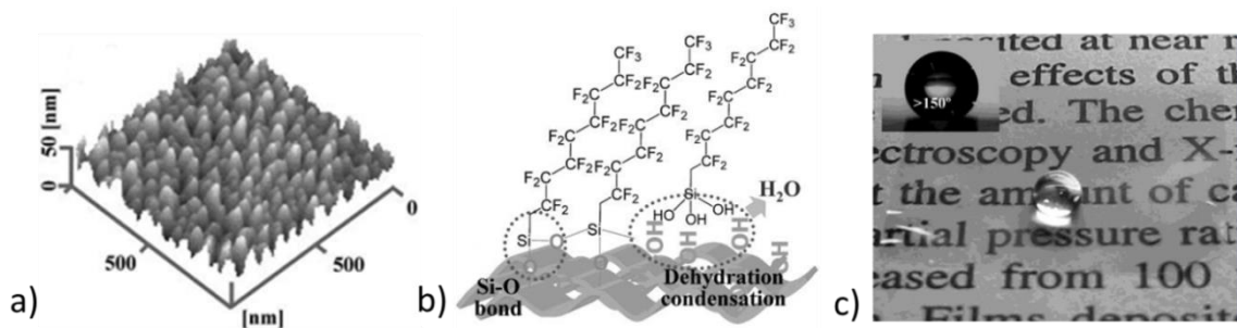
Figure 1.7: (a) Atomic force microscopy (AFM) shows a high density of nanohair structures on the PET surface after anisotropic oxygen plasma etching. (b) Hydrophobization of the nanostructured surface by CVD of semi-fluorosilanes (c) Photographs of water droplets on the transparent superhydrophobic PET substrate after surface hydrophobization. 99
