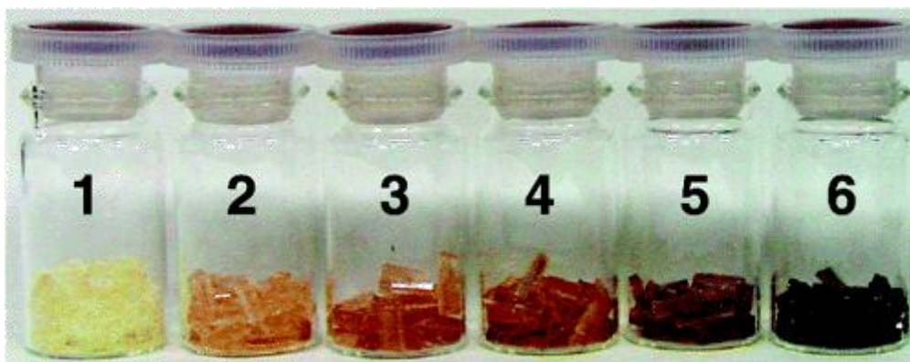
Figure I-2. Appearance of gels containing fractionated clusters of different sizes: \text{Au}_{18}(\text{GSH})_{11} , \text{Au}_{21}(\text{GSH})_{12} , \text{Au}_{25}(\text{GSH})_{14} , \text{Au}_{28}(\text{GSH})_{16} , \text{Au}_{32}(\text{GSH})_{18} and \text{Au}_{39}(\text{GSH})_{23} , labelled as 1-6 respectively. Reprinted with permission from reference 9. Copyright 2004 © American Chemical Society.
