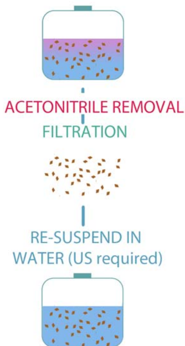
Figure 3.20: Removal of the excess of acetonitrile from NP microsuspensions by filtration. The application of 10 min of US are required to re-dispersed NP micro particles in pure water.
