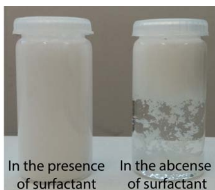
Figure 3.33: Macroscopically comparison between the suspension of ibuprofen in the presence (a) and in the absence of surfactant (b).
