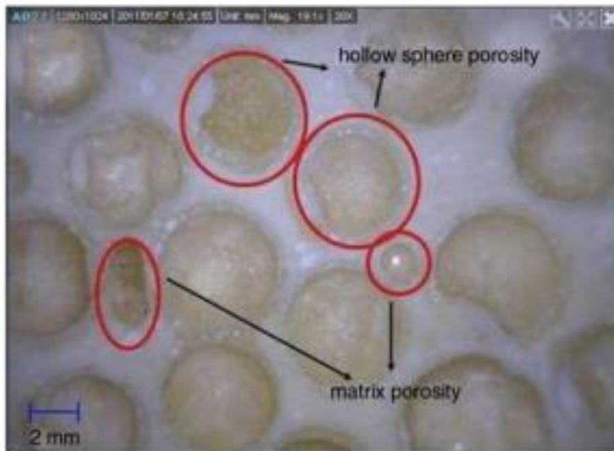
Figure 1.5 Micrograph of syntactic foam containing hollow epoxy microspheres as the fillers [27].
