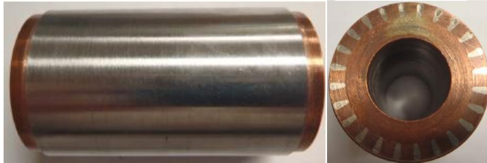
Fig 2.4 Cylindrical rotor design of a high speed induction machine [40]
