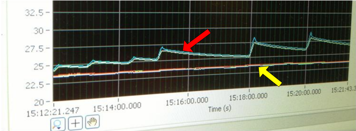
Fig 5.14 Temperature of the SRM prototype with the enhanced rotor at 50 krpm
