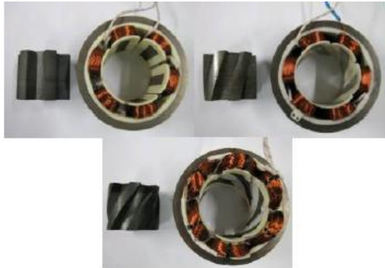
Fig 2.9 A 6/6 SRM prototype with different skew angles (0°; 30°; 64°) [47]
