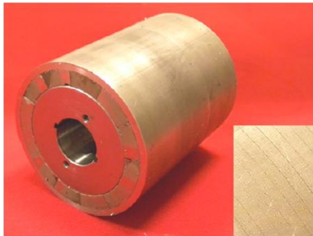
Fig 2.5 Rotor sleeve for a high speed PM machine [41]
