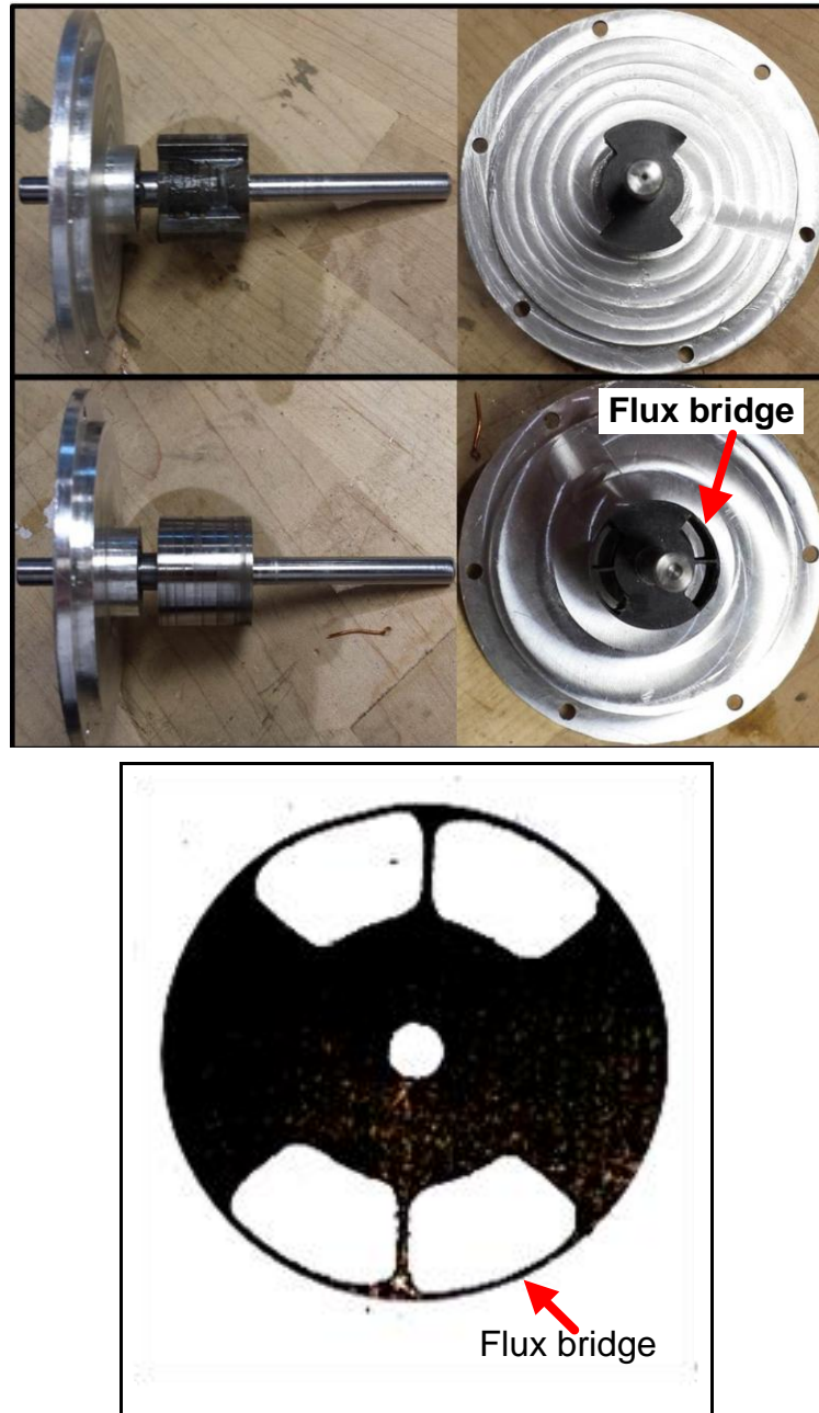
Fig 5.5 Photograph of the prototype motor: rotor (top), lamination (bottom)
