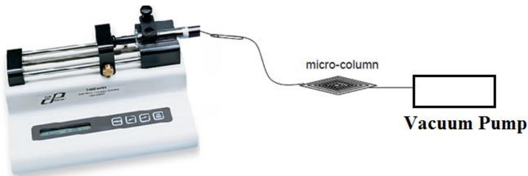
Figure 1-4: Static coating setup
