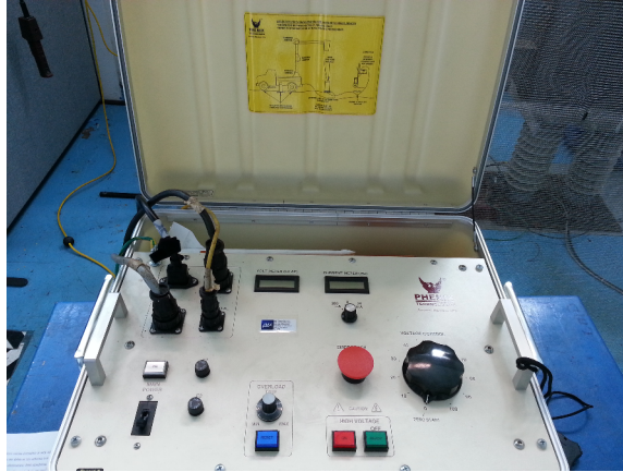
Figure 58: Phenix BK130 high-voltage test set transformer control box.
