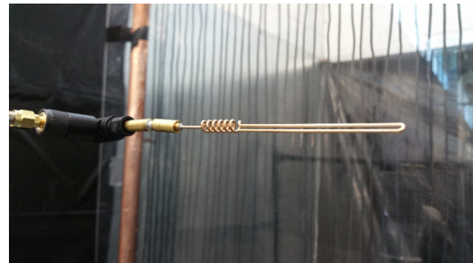
(f) Whip antennas, parallel
