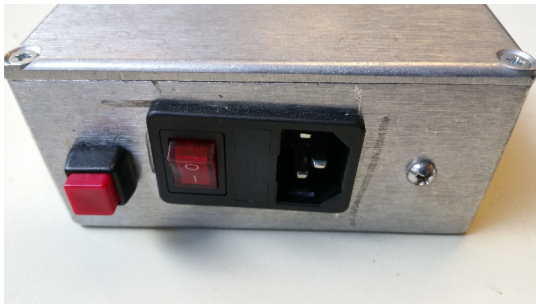
(a) Fused power plug and button
