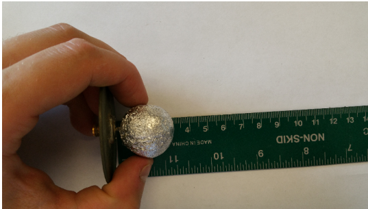
(a) 2.6 cm metal sphere monopole
