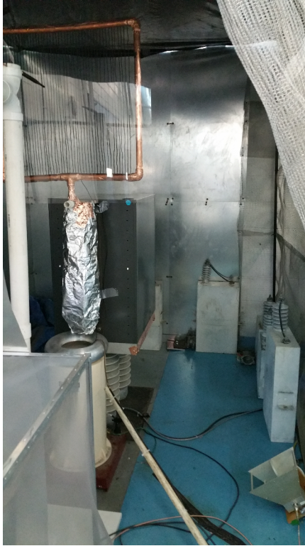
Figure 112: Setup of antenna under test and second measurement antenna (ridged horn on floor) for performing transmission measurements with azimuthal directivity.
