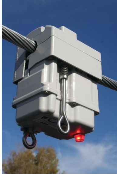
Figure 2: MM3 Line Monitor from Sentient Energy, Inc., rated up to 35 kV [90] for remote power line monitoring.
