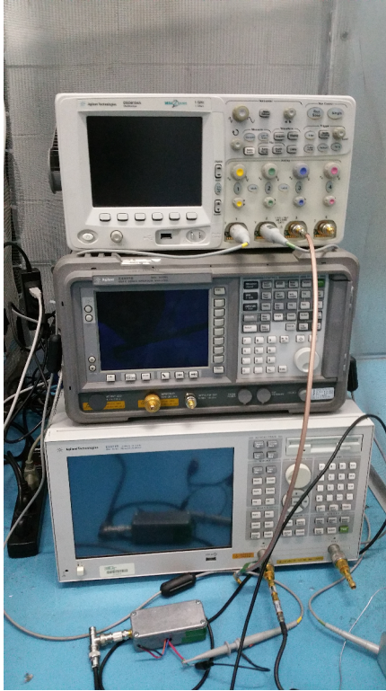
Figure 48: Instruments used in high-voltage antenna experiments. From top to bottom: Agilent Digital Oscilloscope, Agilent Spectrum Analyzer, Agilent Vector Network Analyzer.
