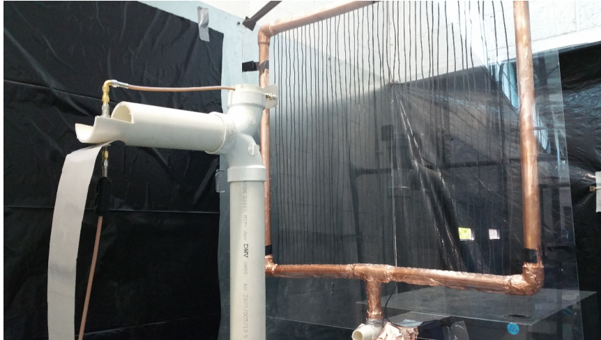
Figure 111: Setup of antenna under test (mounted on PVC stand) and second measurement antenna (patch taped to far wall on right edge of picture) for performing transmission measurements with forward directivity. The antennas are cross polarized with the wire grid.
