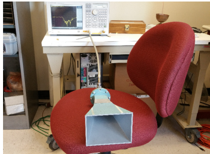
(a) Baseline horn RL measurement
