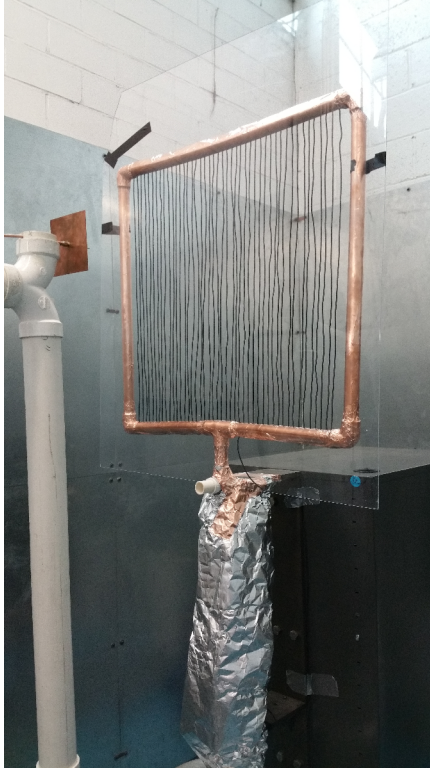
Figure 59: High-voltage plane used to induce corona on the proximate antenna in an inverted voltage setup.
