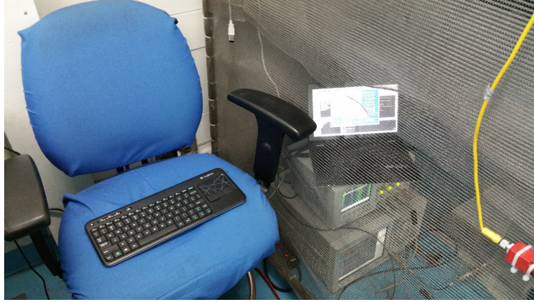
Figure 76: Instrument control setup during measurements. A laptop running MATLAB communicates with the instruments via USB. The laptop is controlled with a wireless keyboard.
