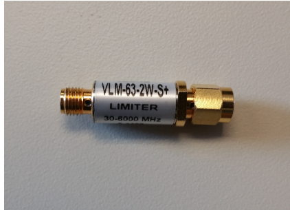
(c) Diode Power Limiter
