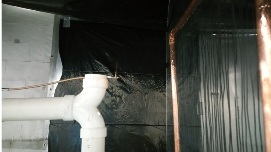
Figure 98: Measurement configuration of the 2.45/5.8 GHz whip antenna. The tip of the antenna is 25 cm from the HV plane.
