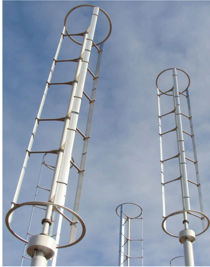
Figure 2.11: A snapshot of Windspire VAWT from Caltech Field Laboratory for Optimized Wind Energy (FLOWE) [1, 2].
