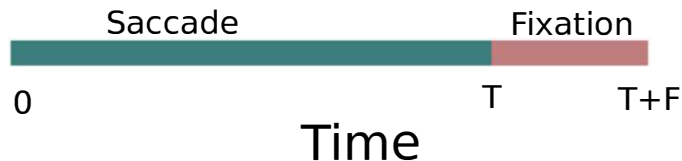
Figure 4.2 The two segments of the finite horizon used for control. First, from time 0 to time T , there is no penalty for the distance from the eye to the target. Second, during fixation (from time T to time T + F ), the penalty on the eye position is enforced. The penalty on the magnitude of the action U is enforced for the entire horizon.
