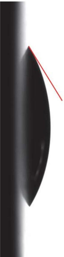
**Figure 3.2:** PC droplet on graphite. Contact angle measurements of 5  $\mu\text{l}$  propylene carbonate drops on a bulk pyrolytic graphite disc (Grade: PG-SN, Graphitstore.com) were performed under ambient conditions using a Rame-Hart contact angle goniometer. The graphite disc was sheared against a paper wipe (Kimwipe) to reveal a fresh surface. The surface was then rinsed with water and allowed to air dry. A static contact angle of  $31.4 \pm 1.6^\circ$  was obtained from 3 trials
