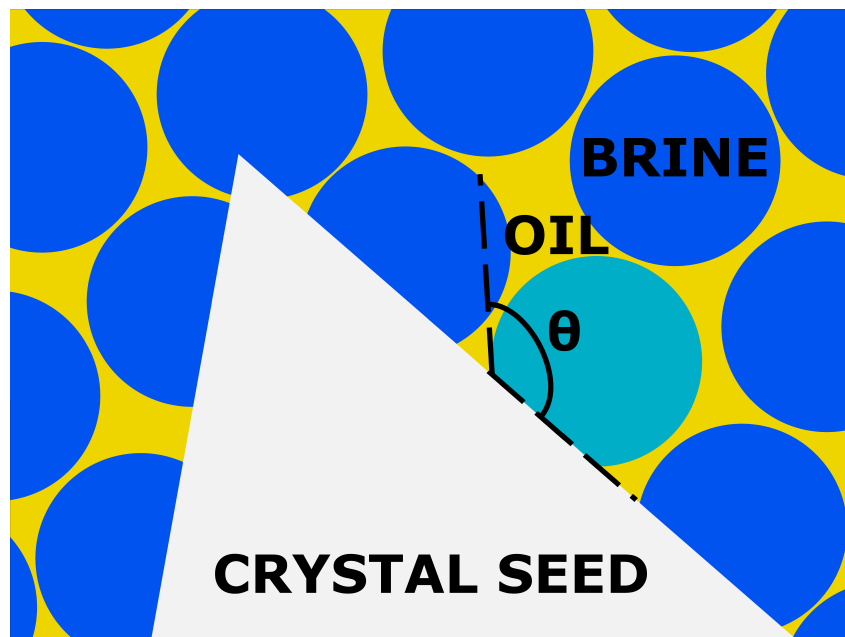
(b) Crystal seed and the droplets in the emulsion; highlighting of one drop is used only to describe the contact angle.
