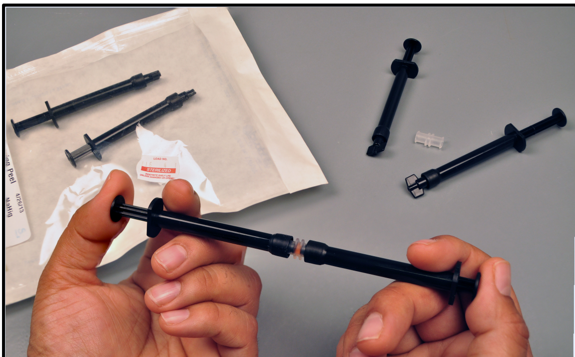
Figure 5.8 Sterile complex coacervate adhesive packets used in the animal studies. One syringe contains the coacervate adhesive and the second the chemical initiator. Upon use, the two solutions are mixed by connecting the two syringes with a mixing nozzle. The adhesive/initiator are mixed by pushing out the matter from one syringe to the other, 5–10 times, or 30 sec. The adhesive is then pushed into one syringe; the empty syringe is removed, with a cannula secured on the leur-lock adhesive syringe, and the adhesive is applied at the site within a minute.
