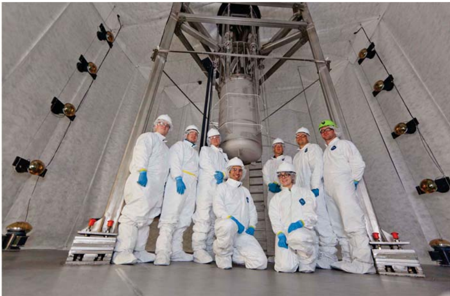
Figure 2.1: Photo of the outer vessel of the LUX detector from inside the water tank.
