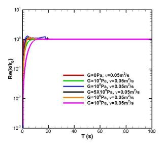
Fig. 8-8 Real part  $\kappa/k_0$  with respect to wave period T. h = 1m, H = 100m.
