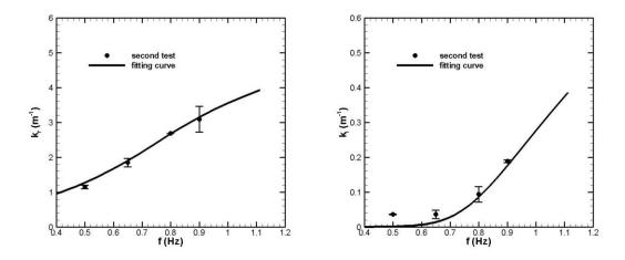
Fig. 6-13 Data fitting by viscoelastic model for the second test using Levenberg–Marquardt algorithm (LMA).  $G = 5.1 \times 10^5 \,\mathrm{Pa}$ ;  $\nu = 61.1 \mathrm{m}^2/\mathrm{s}$ .
