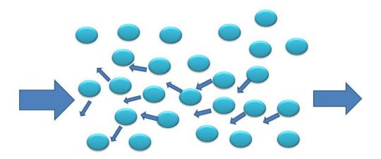
Fig. 2-3 Sketch of the scattering mechanism: large left arrow represents incident wave; large right arrow represents transmission wave; small arrows represent reflected waves; particles represent ice floes.
