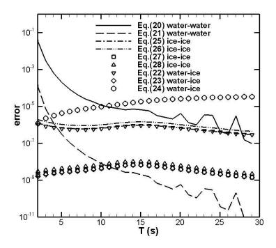
Fig. 4-16 Error terms from different boundary conditions:  $G_1 = G_3 = 5$ GPa,  $v_1 = v_3 = 0$ m<sup>2</sup>/s,  $h_1 = 1$ m,  $h_3 = 2$ m and H = 100m.
