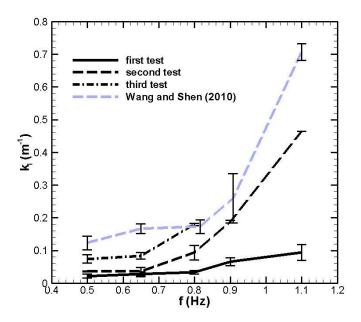
Fig. 6-9 Wave attenuation with respect to wave frequency.
