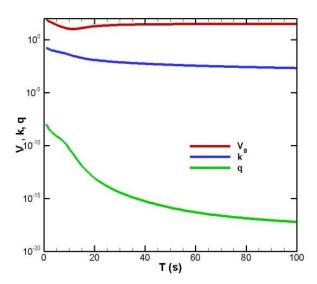
Fig. 8-7 Real part  $\kappa$  and imaginary part q and group velocity  $V_g$  with respect to wave period T.  $v_{ice} = 0.05 m^2/s$ ,  $G = 10^9 Pa$ . h = 1m, H = 100m.
