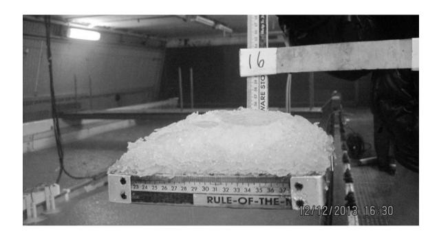
Fig. 6-4 Mesh-scoop ice sampling. One pancake is shown lying on top of the slushy ice accumulation. The stick label shows the sample is picked up at the 16m mark location along the tank.
