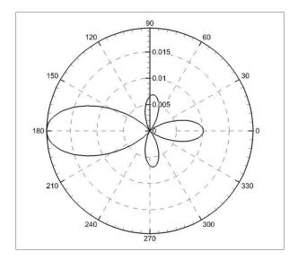
Fig. 2-4 The scattered wave energy plotted in polar coordinate for 100m waves scattered by a circlar ice floe. The ice thickness is 1m. The floe diameter is 50m, and its Young's modulus is 6GPa. (Reproduced by Sukun Cheng following Meylan.)
