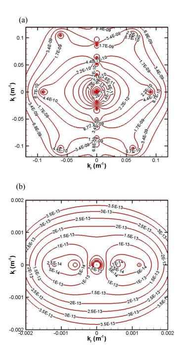
Fig. 5-2 Contour lines of the residual function abs(Det). Here  $v = 0\text{m}^2/\text{s}$ , G = 1GPa, and h = 0.5m. (a) Wide-angle view where evanescent modes, two damped traveling modes, and the third mode on the real axis is seen near  $k_r = 0.1\text{m}^{-1}$ ; (b) Close-up view where the two modes on the real axis are seen.
