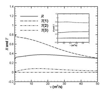
Fig. 5-6 Reflection and transmission coefficients with respect to viscosity between open water and viscous ice with  $h_1 = 0$ m,  $h_3 = 0.5$ m,  $G_3 = 0$ Pa, and T = 6s.
