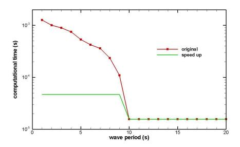
Fig. 8-9 Computational time with respect to wave period for original method and speed up method.
