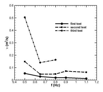
Fig. 6-11 Effective viscosity with respect to wave frequency by inverse method.
