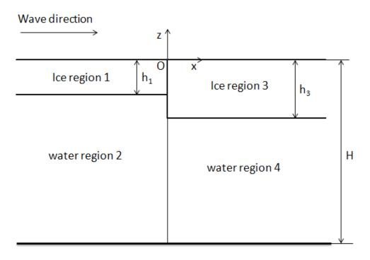
Fig. 4-3 Schematic of the coordinate frame of the problem.
