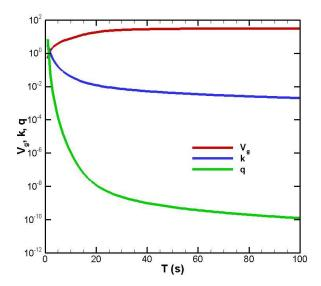
Fig. 8-2 Real part  $\kappa$  and imaginary part q and group velocity  $V_g$  with respect to wave period T.  $v_{ice}=0.05m^2/s$ , G=0Pa.h=1m, H=100m.
