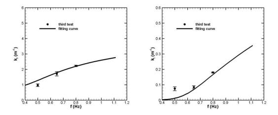
Fig. 6-14 Data fitting by viscoelastic model for the third test using Levenberg–Marquardt algorithm (LMA).  $G = 1.0 \times 10^6 \,\mathrm{Pa}$ ;  $\nu = 139.3 \,\mathrm{m}^2/\mathrm{s}$ .
