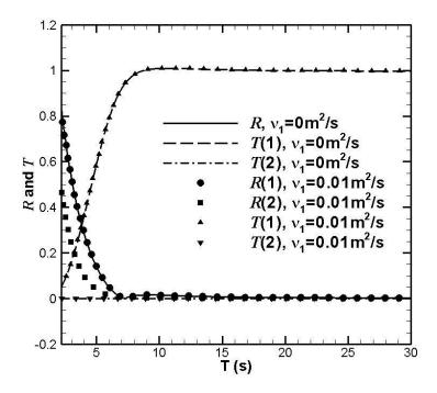
Fig. 4-14 Reflection and transmission coefficients with respect to wave period from open water or a pure viscous ice to a pure elastic ice with  $G_1$ =0Pa,  $v_1$ =0m²/s or 0.01m²/s,  $G_3$ =0.05GPa,  $v_3$ =0m2/s, and  $h_1$ =1m,  $h_3$ =1m.
