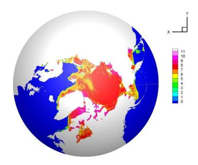
Fig. H-2 computed effective viscosity of Arctic ice cover in log scale.
