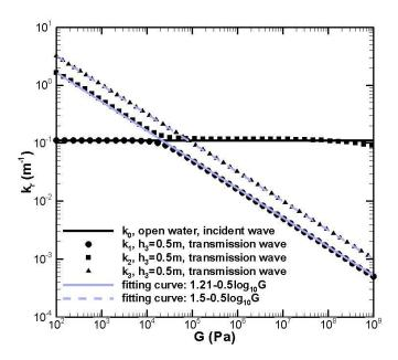
Fig. 5-7 Wave number of pure elastic ice with  $v_3 = 0$ m<sup>2</sup>/s, T=6s and  $h_3 = 0.5$ m, H = 100m.
