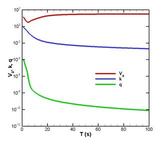
Fig. 8-5 Real part  $\kappa$  and imaginary part q and group velocity  $V_g$  with respect to wave period T.  $v_{ice} = 0.05m^2/s$ ,  $G = 5 \times 10^5 \, Pa$ . h = 1m, H = 100m.
