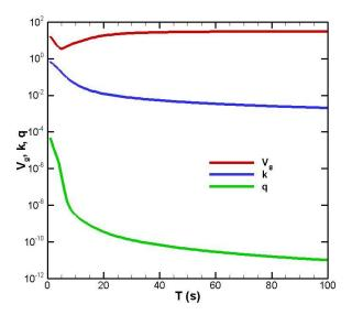
Fig. 8-6 Real part  $\kappa$  and imaginary part q and group velocity  $V_g$  with respect to wave period T.  $v_{ice} = 0.05 m^2/s$ ,  $G = 10^6 Pa$ . h = 1m, H = 100m.
