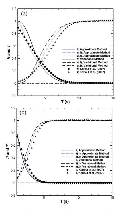
Fig. 5-1 Comparison between previous and the present studies of the reflection and transmission coefficients from open water to an elastic cover with respect to wave period. Here  $\nu = 0 \text{m}^2/\text{s}$  for both regions,  $h_1 = 0 \text{m}$ ,  $G_3 = 1 \text{GPa}$ , and (a)  $h_3 = 0.5 \text{m}$ ; (b)  $h_3 = 0.1 \text{m}$ . In this and the rest of the figures,  $\rho_{ice} = 917 kg/m^3$ ,  $\rho_{water} = 1000 kg/m^3$ . (The dark and grey dash-dot lines coincide.)
