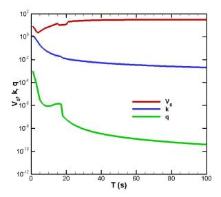
Fig. 8-4 Real part  $\kappa$  and imaginary part q and group velocity  $V_g$  with respect to wave period T.  $v_{ice} = 0.05 m^2 / s$ ,  $G = 10^5 Pa.h = 1m$ , H = 100m.
