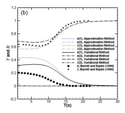
Fig.5-4 Reflection and transmission coefficients with respect to wave period between two elastic ice regions with  $v = 0\text{m}^2/\text{s}$  in both regions. (a)  $G_1 = 2\text{GPa}$ ,  $G_3 = 5\text{GPa}$ , and  $h_1 = h_3 = 1\text{m}$ ; (b)  $G_1 = G_3 = 5\text{GPa}$ ,  $h_1 = 1\text{m}$ ,  $h_3 = 2\text{m}$ . (In both cases, R(2) and R(2) are zero for both approximate method and variational method.)
