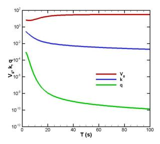
Fig. 8-3 Real part  $\kappa$  and imaginary part q and group velocity  $V_g$  with respect to wave period T.  $v_{ice}=0.05m^2/s$ ,  $G=10^4Pa$ . h=1m, H=100m.
