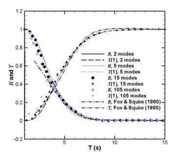
Fig. 5-3 Effect of including additional modes on transmission/reflection from open water to an elastic sheet with the same parameters as in Fig.7-1 (2 modes: include 2 propagating modes; 5 modes: add 1 additional propagating mode and 2 symmetrical damped propagating modes; 15 modes: add 10 evanescent modes to the 5 modes case. 105 modes: add 100 evanescent modes to the 5 modes case. Fox and Squire's results used 100 evanescent modes. Sukun Cheng reproduced Fox and Squire's results.)
