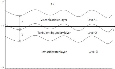
Fig. 3-1 The sketch of the three-layer viscoelastic model.
