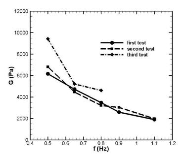
Fig. 6-10 Effective shear modulus with respect to wave frequency by inverse method.
