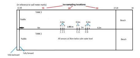
Fig. 6-1 Basin configuration and pressure transducer locations.
