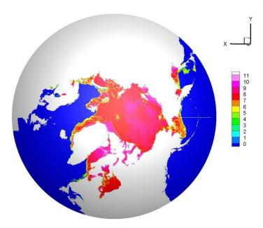
Fig. H-1 computed effective elasticity of Arctic ice cover in log scale.
