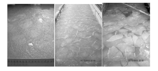
Fig. 6-3 (Left) Frazil/pancake ice mixture with a meter stick shown at the bottom of the photo. (Center) Pancake ice. (Right) Fragmented ice floe.
