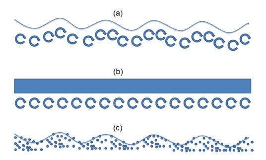
Fig. 2-2 Three mechanisms for viscous attenuation: (a) turbulence in the upper layer of the ocean; (b) boundary layer flows under ice cover; (c) interactions of ice particles.
