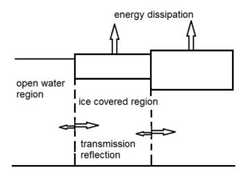
Fig. 4-1 Schematic of a discretized field of wave propagation into a continuous heterogeneous ice cover.
