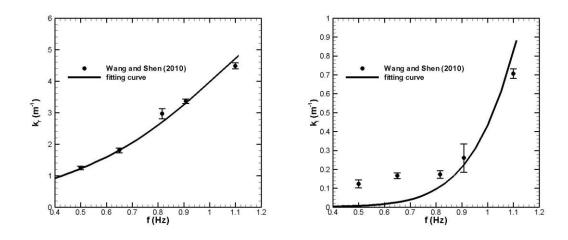
Fig. 6-15 Data fitting by viscoelastic model for Wang and Shen (2010a) using Levenberg–Marquardt algorithm (LMA). G = 48.24 Pa;  $\nu = 0.04 \text{m}^2/\text{s}$ .
