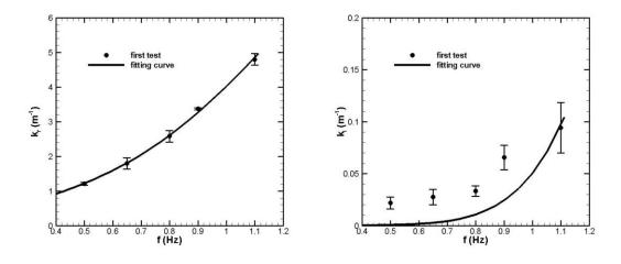
Fig. 6-12 Data fitting by viscoelastic model for the first test using Levenberg–Marquardt algorithm (LMA). G = 21Pa;  $\nu = 0.014\text{m}^2/\text{s}$ .
