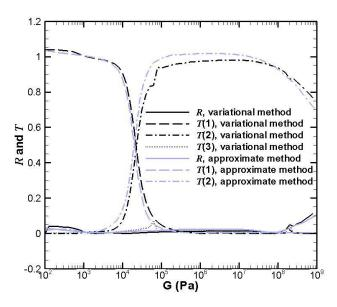
Fig. 5-5 Reflection and transmission coefficients with respect to shear modulus between open water and elastic ice with  $h_1 = 0$ m,  $h_3 = 0.5$ m,  $v_3 = 0$ m<sup>2</sup>/s, and T = 6s.
