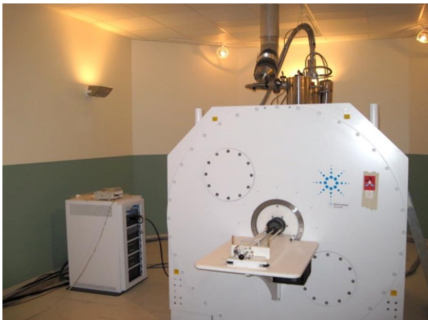
Figure 6.4. Agilent 9.4 T MRI scanner.
