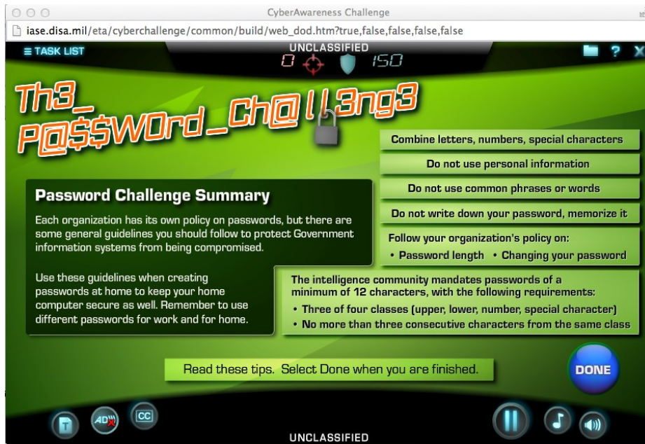
Figure 9. Th3 P@$$WOrd_Ch@ll3ng3 summary screen showing the mandatory password complexity policy used in the intelligence community (DISA, 2013).
