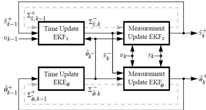
Figure 2.6: Diagram of dual EKF. (Courtesy of [67].)
