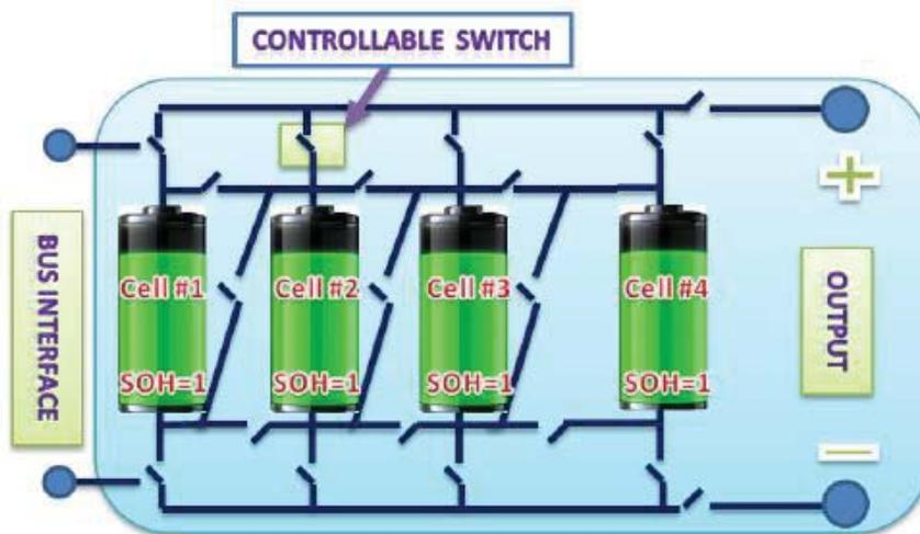
Figure 2.2: A reconfigurable multicell battery topology. (Courtesy of [21].)
