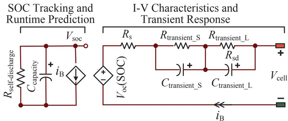
Figure 2.3: An electrical circuit battery model. (Courtesy of [42].)
