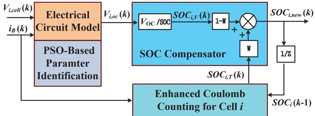
Figure 5.2: The proposed closed-loop weighting SOC estimation algorithm.
