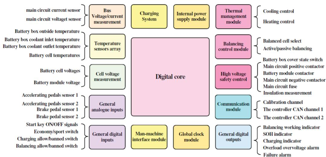
Figure 2.1: Framework of a typical BMS. (Courtesy of [6].)
