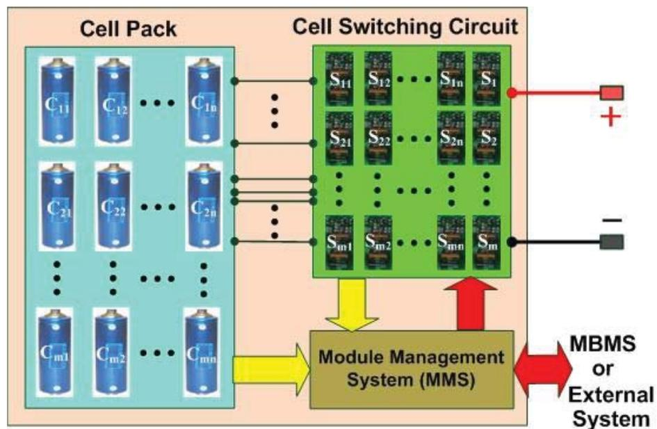
Figure 4.1: The self-X, multicell battery module design.
