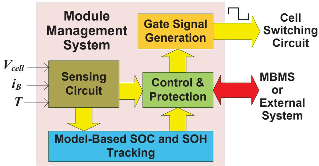
Figure 4.5: Schematic diagram of the module management system.
