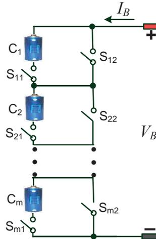
Figure 4.12: The proposed series-connected, self-reconfigurable, multicell battery topology.
