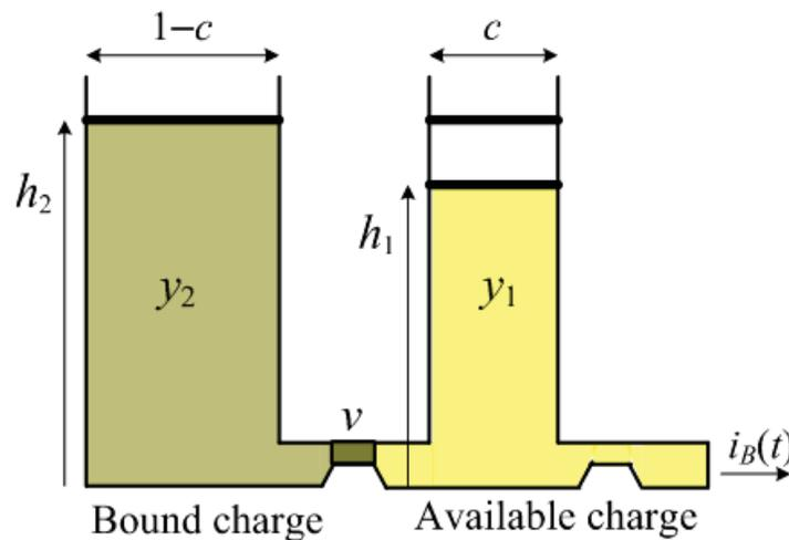
Figure 2.4: The kinetic battery model. (Courtesy of [49].)
