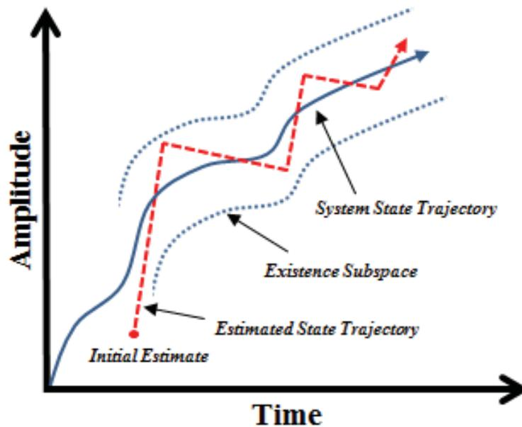
Figure 7.2: The SVSF estimation concept. (Courtesy of [112].)
