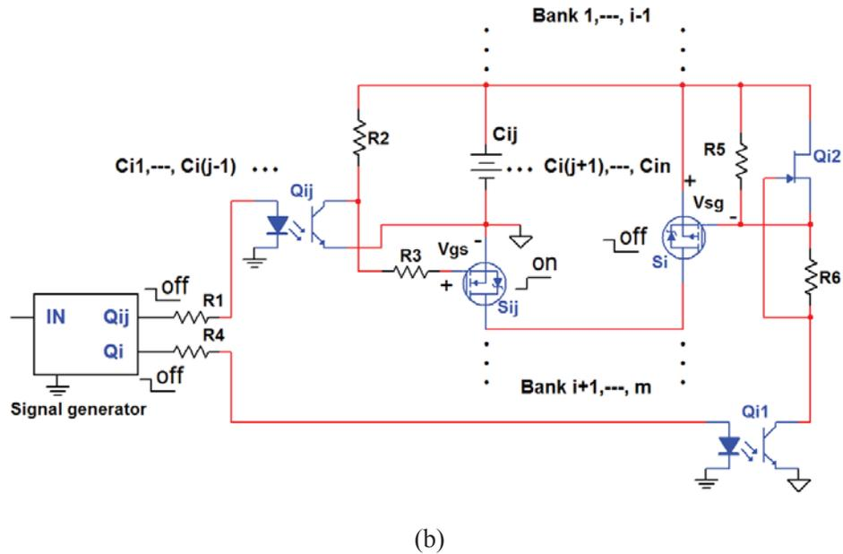
Figure 4.3: Switch implementation for Cell  $C_{ij}$  using an n-channel power MOSFET and for Bank  $i$  using a p-channel power MOSFET with a gate drive circuit using (a) small-signal BJTs and (b) optocouplers.
