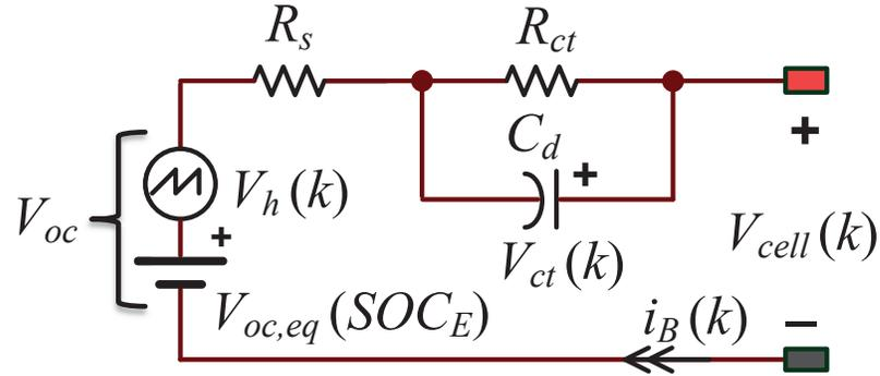
Figure 3.13: The electrical circuit with hysteresis battery model.
