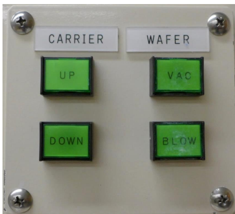
Figure 2.3: Manual switches on the front side of the APD-800.
