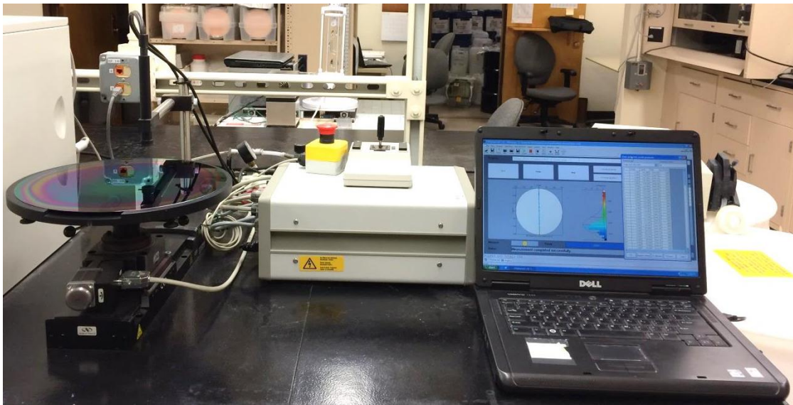
Figure 2.23: SENTECH FTP reflectometer.
