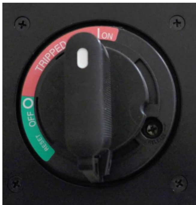
Figure 2.2: The primary ON/OFF switch of the APD-800.
