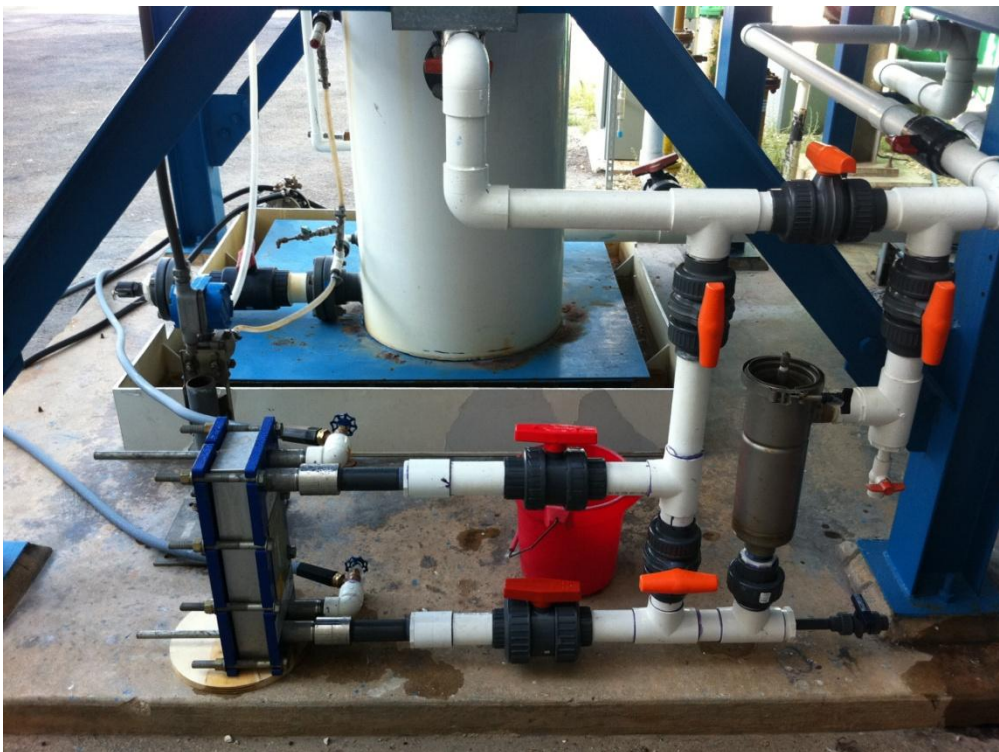
Figure A.9: Chilled water cooling system
