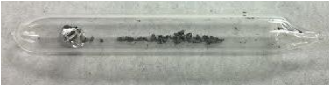
Figure 111: Post reaction quartz vessel with a large arsenic crystal and boron substrates that had visibly undergone a reaction.
