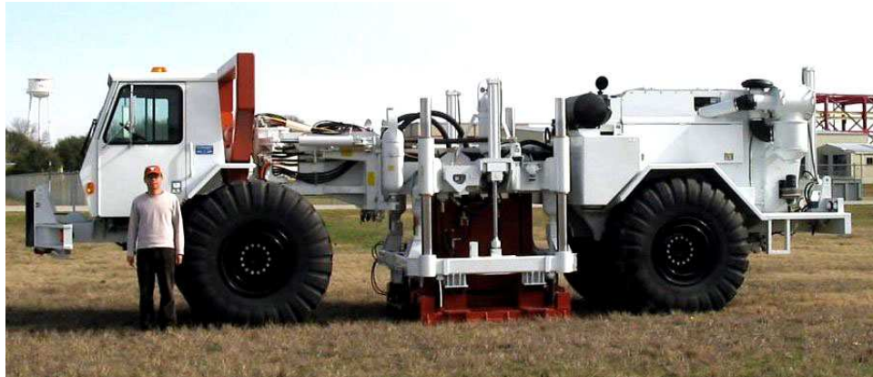
Figure 4.8: NEES@UTexas Liquidator Vibroseis.
