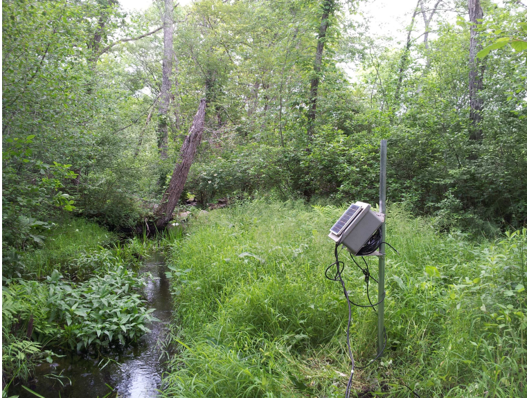
Figure 4.8: Image showing the waterproof housing at Forest 1 that contains the battery and datalogging equipment. The solar panel is mounted on the outside of the housing
