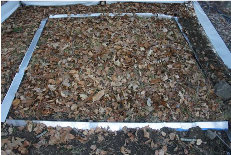
Figure 2.8: Forest study site, showing aluminum flashing. The collection point is at the lower right corner. The aluminum flashing on the right and bottom sides of the picture are the runoff channels. Due to the slope from the top left to the bottom right, the aluminum flashing on the left and top sides only isolate the plot and do not carry water to the collection point
