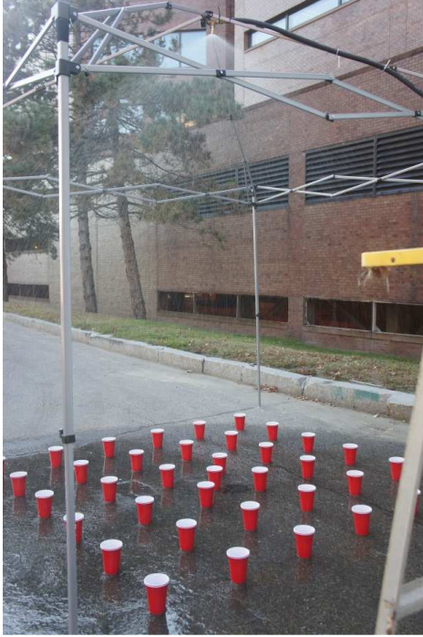
Figure 2.2: Rain simulator in operation during drop dispersion testing
