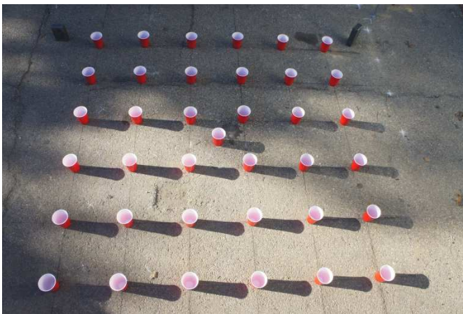
Figure 2.4: 2 by 2 meter grid with cups spaced at 0.4 meter intervals
