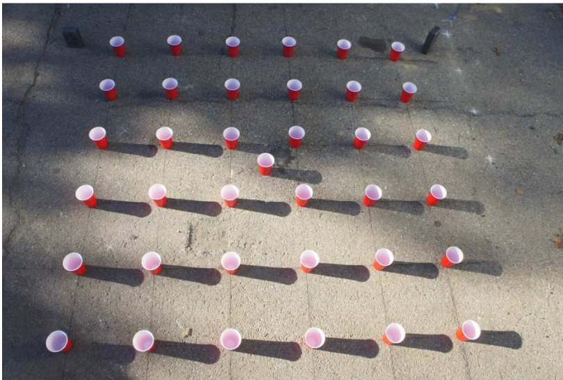
Figure 3.4: 2 by 2 meter grid with cups spaced at 0.4 meter intervals
