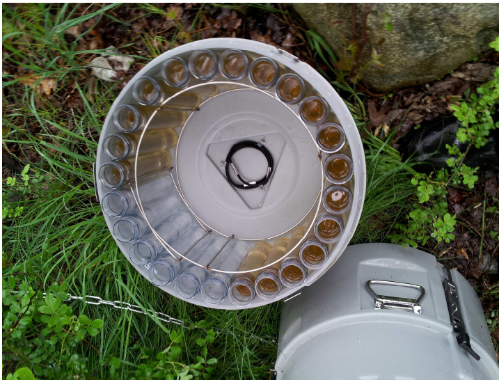
Figure 4.9: Interior of autosampler sample chamber with samples collected during a storm event
