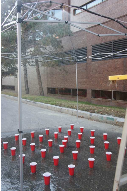
Figure 3.5: Rain simulator in operation during drop dispersion testing
