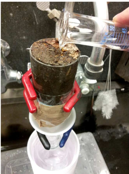
Figure 3.10: Soil column setup for infiltration testing
