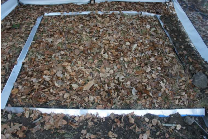
Figure 3.9: Forest study site, showing aluminum flashing. The collection point is at the lower right corner. The aluminum flashing on the right and bottom sides of the picture are the runoff channels. Due to the slope from the top left to the bottom right, the aluminum flashing on the left and top sides only isolate the plot and do not carry water to the collection point
