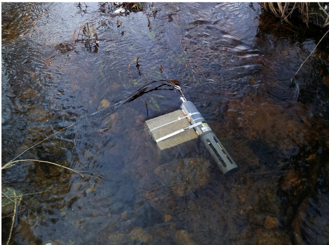
Figure 4.7: YSI sonde deployed at Forest 1. The sonde is mounted on a cinder block. The fluorometer is mounted below the YSI sonde and not visible in this picture
