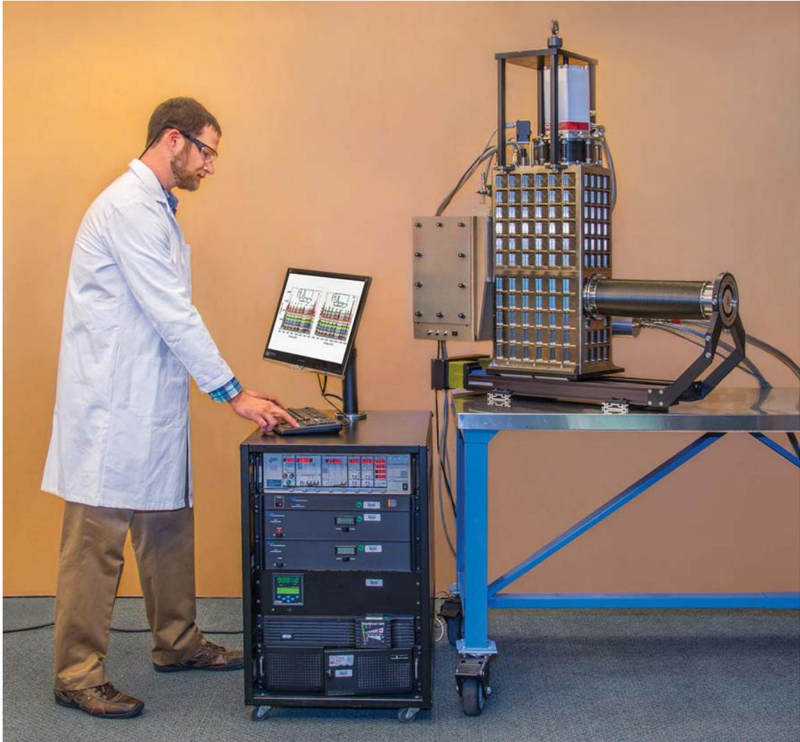
Figure 6.3: The author analyzes high-resolution x-ray spectra with the STJ detector.
