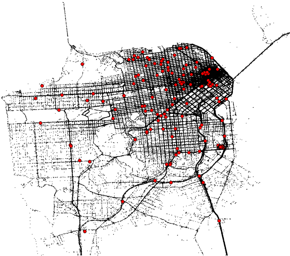
Figure 1.2.1: An example of dataset available to Mobile Millennium [20] and processed by the path inference filter [63]: taxicabs in San Francisco from the Cabspotting program [10]. Large circles in red show the position of the taxis at a given time and small dots (in black) show past positions (during the last ten hours) of the taxi fleet. The position of each vehicle is observed every minute.
