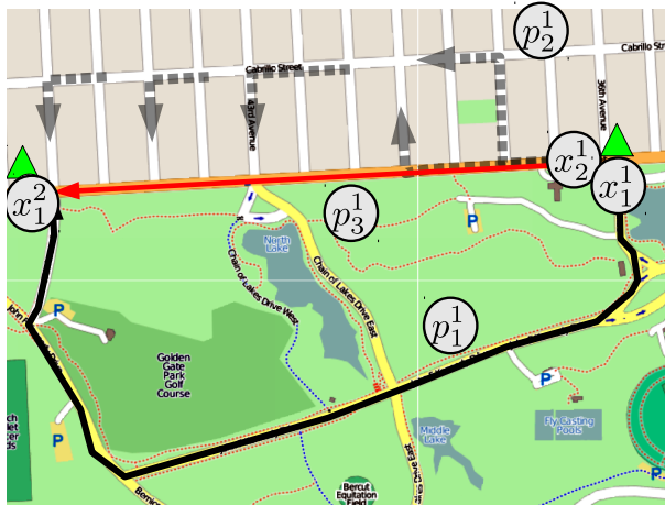
Figure 2.3.3: Example of a failure case when using a Hidden Markov Model: the solid black path will be favored over all the other paths. The paths p_i^1 connect the states x_j^1 to x_k^2 . See section II for more details on the notations.
