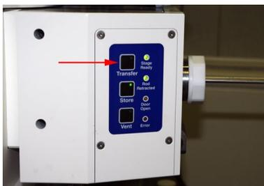
7. Once the gate valve is open fully, push the sample holder into the chamber by pushing on the white teflon disk mounted on the specimen exchange rods. Watch as the sample holder mates with its corresponding dovetail on the stage. Make sure the sample holder is on the dovetail and pushed completely on the stage.
