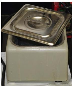
3. Immediately after removing the silicon from the Acetone, place in Isopropyl Alcohol (IPA), as Acetone tends to leave residue on the surface as it dries.
