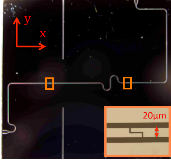
Figure 6.4: CPWR used for strong coupling a scanning transmon qubit. Inset shows finger capacitors used to define the photon escape rate \kappa = 10 MHz. Subsequent qubit positions follow the x and y coordinate system shown here.
