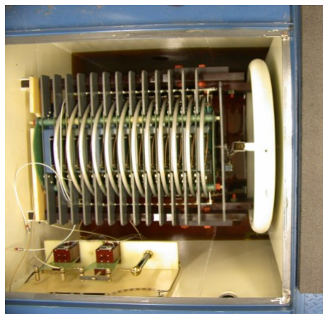
Figure 30. The NOTES Legacy 24 stage Marx Generator
