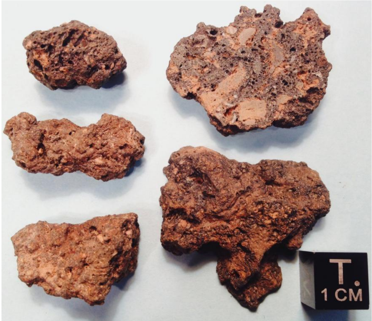
Figure 4.3. Scoriaceous impact glass from the Monturaqui (left) and Henbury (right) impact craters. Impact glasses have been found at 8 of the 22 sub-km crater locations, and have proven to be an effective research target for locating unambiguous impact evidence including metal spherules, indicative elemental ratios, and formation of planar deformation features, diaplectic glass, and high pressure mineral polymorphs in trapped mineral grains.
