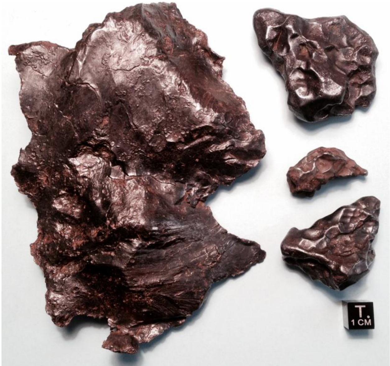
Figure 4.2. Left: An example of shrapnel specimen from the Sikhote Alin meteorite, exhibiting characteristic torn appearance and sharp edges. Macroscopic plastic deformation of shrapnel fragments is typically accompanied, internally, by distorted crystallographic structure, the formation of shear surfaces, brittle failure on inclusion and crystal boundaries, and evidence of transient localized re-heating. Right: Individuals from the same fall, showing clear regmaglypts.
