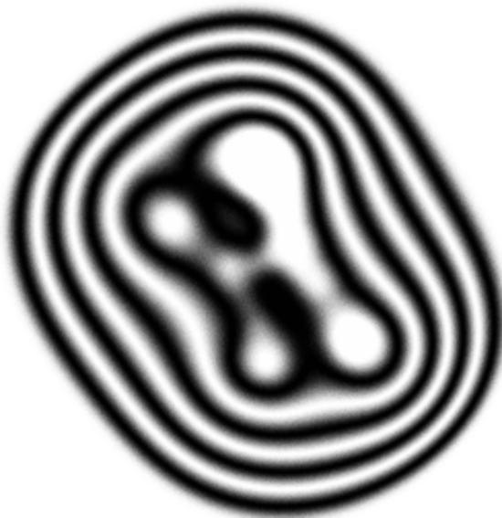
Figure 6.5: The implicit field created using a thin plate spline multiplied by a cosine function.
