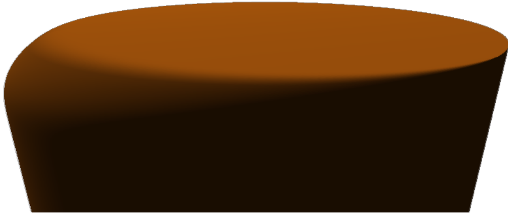
Figure 5.1: Interpolation between a straight edge along a cylinder top cap (right) and its filleted version (left).
