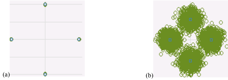
Figure 10. (Left) Signal constellation without ASE. (Right) Signal constellation with ASE
