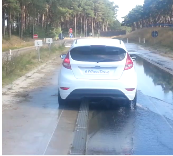
Figure 4.5.1: Experimental Vehicle with Wheel-Motors Installed at Each Rear Wheel, Being Tested on a Slip- \mu Surface
