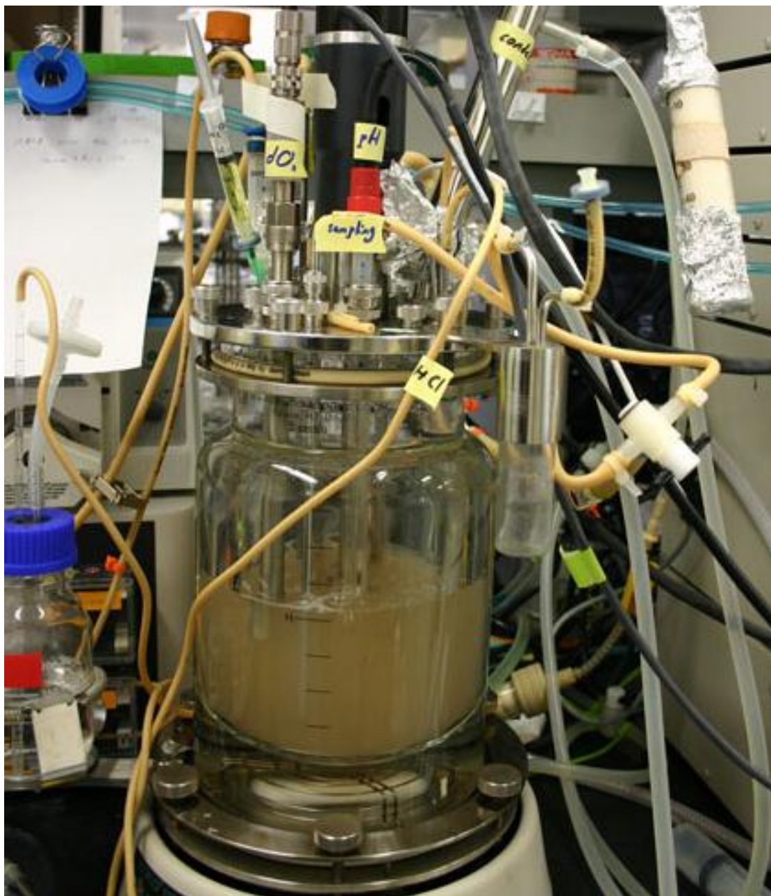
Figure 4.9: Picture of a chemostat used for analyzing the expression levels of various genes before and after production of bacterial nanowires by S. oneidensis MR-1 cells.
