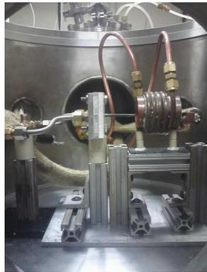
Figure 4.31: Solid cathode assembly under an experiment [2].
