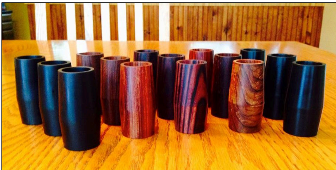
Figure 14. Finished 66-Millimeter Barrels Used in Pilot Study. From Left to Right: Grenadilla, Mopane, Purpleheart Wood, Cocobolo, and Delrin.
