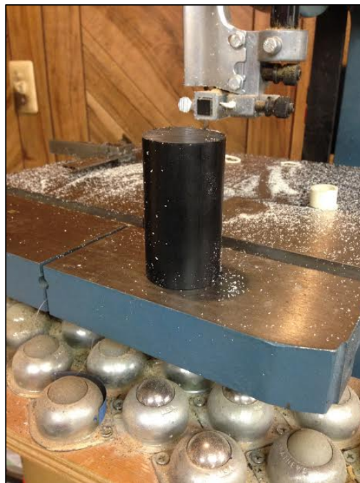
Figure 4. Delrin after Being Reduced to 3" in Length
