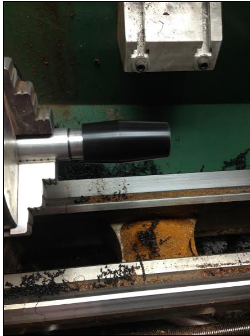
Figure 11. Barrel after Completion of Top and Bottom Exterior Contouring and Respective Tenon Measurements.
