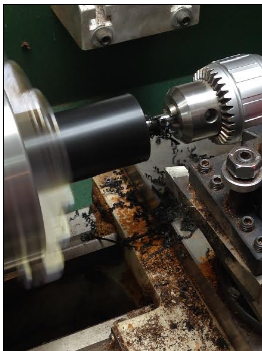
Figure 5. Delrin Receiving Rough Bore.
