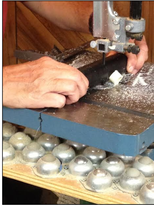
Figure 3. Delrin is Cut to 3" in Length.
