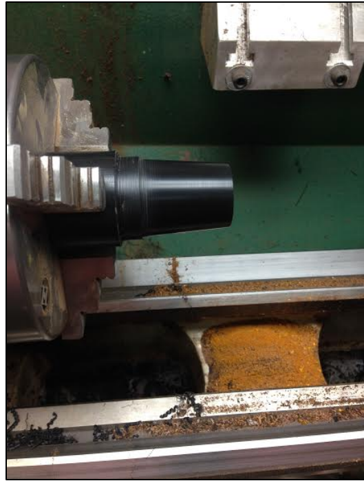
Figure 9. Barrel after Being Contoured
