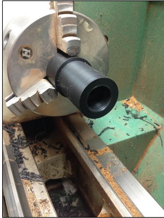
Figure 7. Barrel after Receiving Appropriate Top Joint Tenon Socket Measurements.
