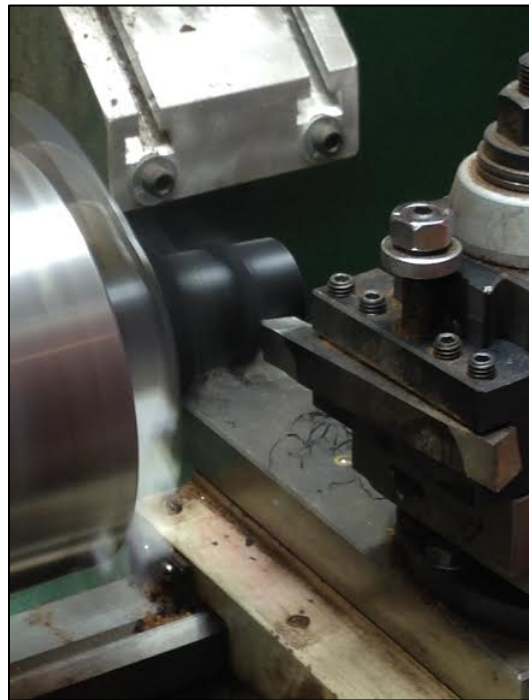
Figure 8. Shaping of Barrel Exterior Contour.
