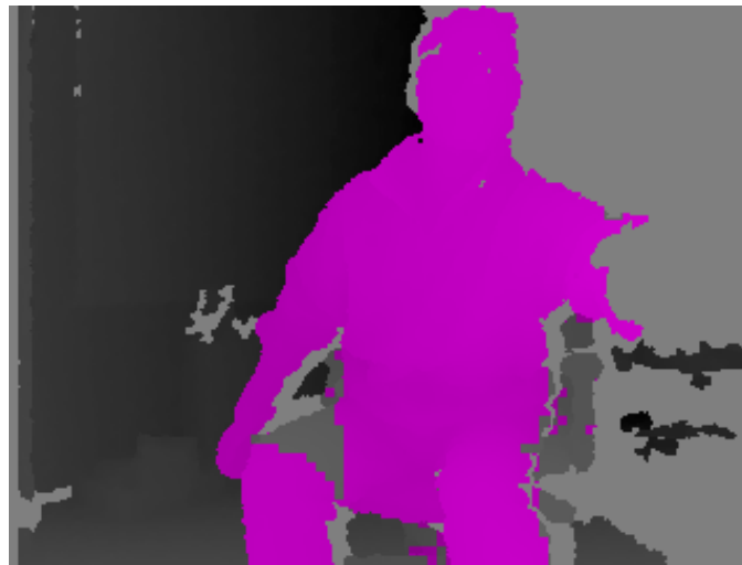
Figure 1.5. Depth map generated by Kinect depth camera
