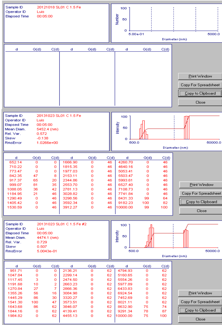
Figure D11. Particle size analysis results for Halomonas sp. SL01 Halochelin C at 1.5 Eq. Fe +3 .
