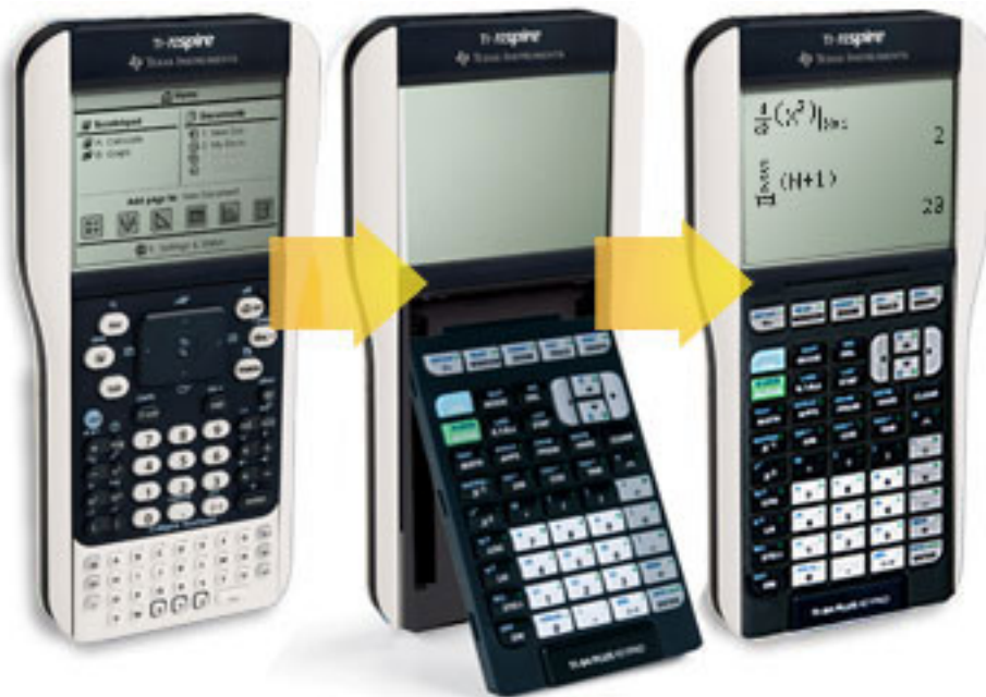
Figure 1.1. Displaying the interchangeable keypads of the TI-Nspire (Texas Instruments, n.d.).
